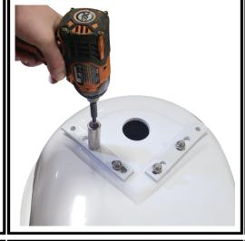
4. Using the supplied bolt & washers; attach the clawfeet to the brackets through the threaded hole on each end of the bracket.
